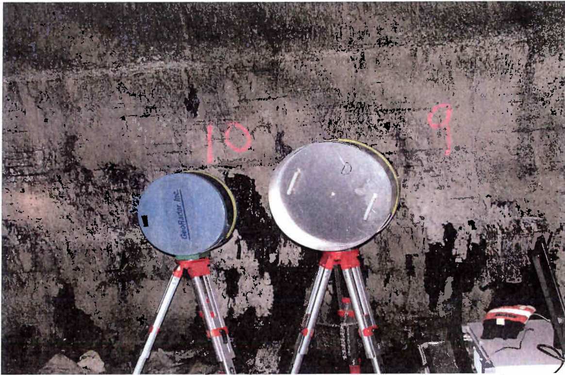
Photo 9: Transmitting and Receiving Antennas for reflection test at Mine 84.
