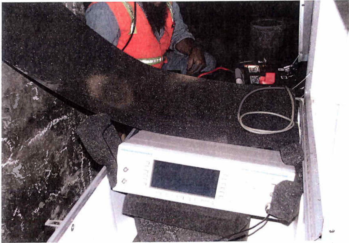
Photo 11: Data collection using commercial signal generator/spectrum analyzer during preliminary testing at Mine 84.
